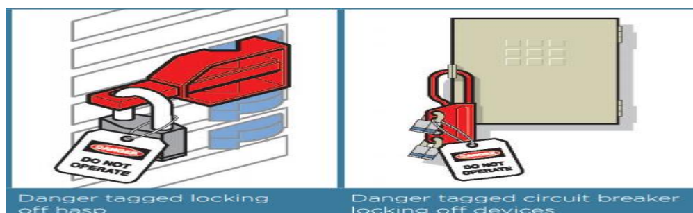
Fig. 6.1 machine/equipment in lockout
