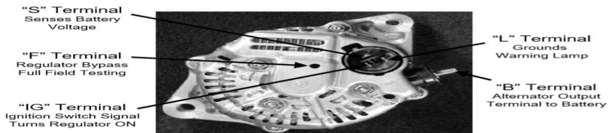
Fig5.16 alternator terminal identification
