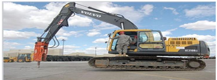
An excavator-mounted hydraulic jackhammer being used to break up concrete.
