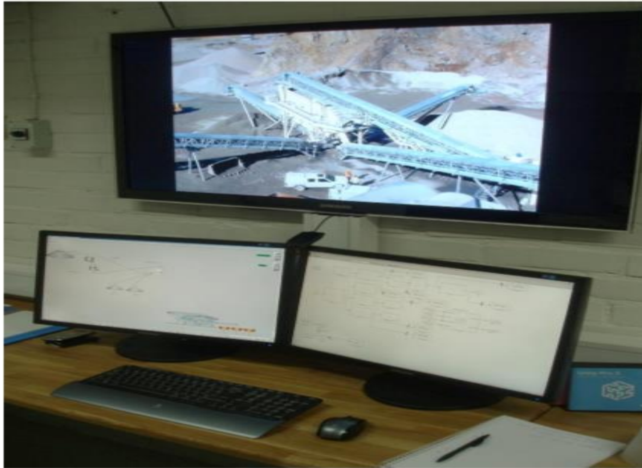
Figure 1: The simulation computer running a plant simulation while information is being transferred to the operator's screen.
