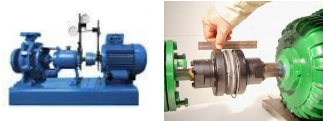
Fig1.5 Motor-pump Alignment using a dial indicator and a straight edge
