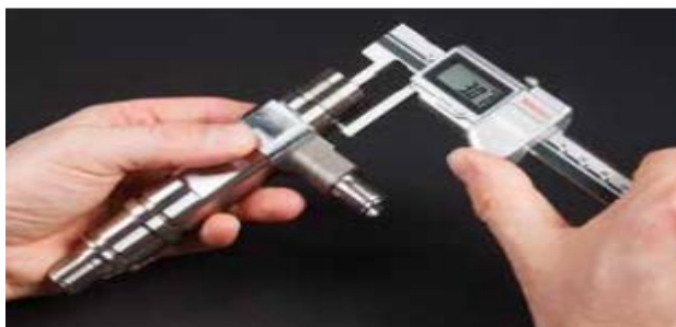
Fig. 2.2. Application of a point jaw caliper
