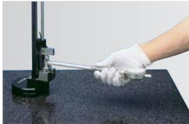
Fig. 2.30. bore gauge checker with gauge blocks
