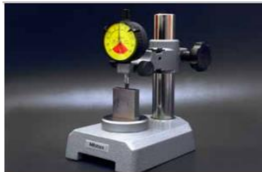
Fig.2.57. Reference point setting with a 50 mm Gauge Block.
