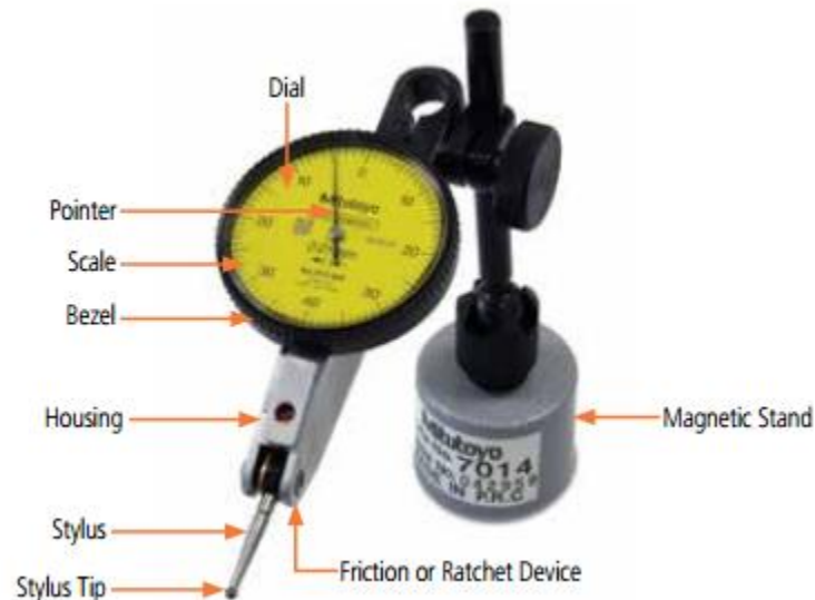
Fig. 2.48. Parts of dial test indicator.
