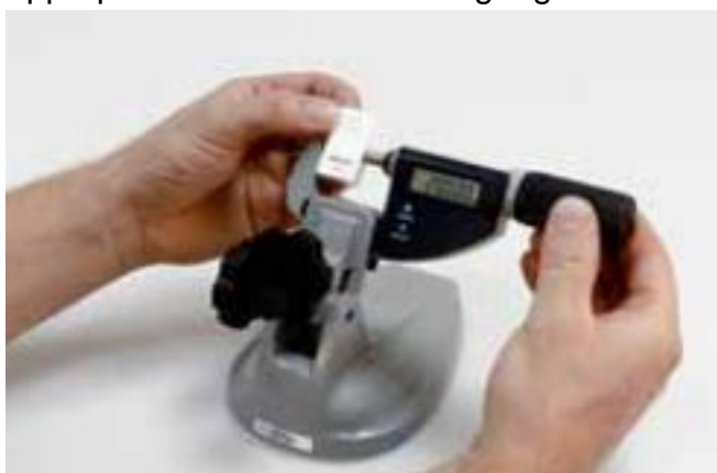
Fig.2.4. Reference point setting with a gauge block
