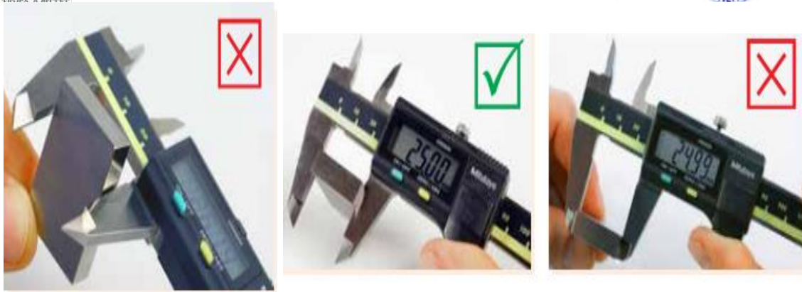
Fig.2.37. correct use of calipers
