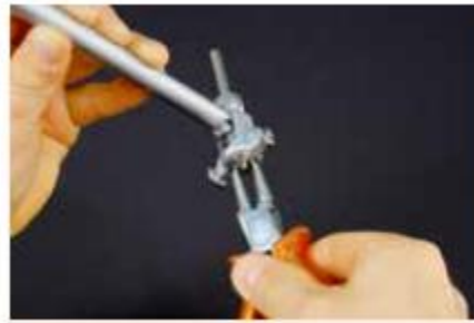
Fig.2.34. film of micrometer oil to the contact point and the driver pin
