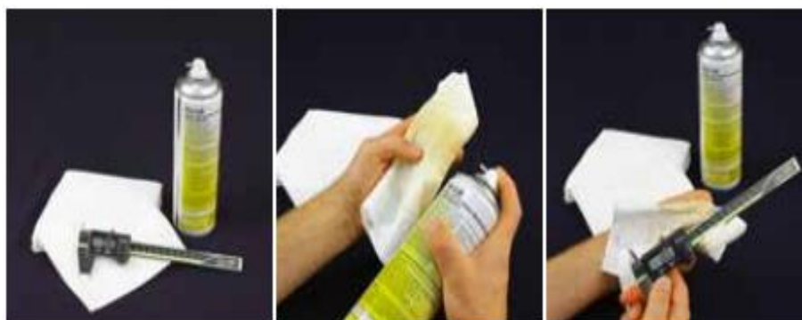
Fig.2.10. apply anti-corrosive coating for rust prevention
