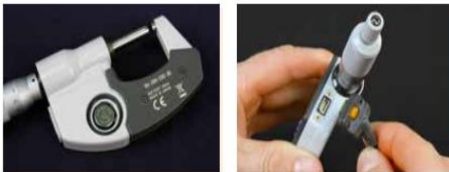
Fig. 2.15. Rubber seal to protect the battery housing
