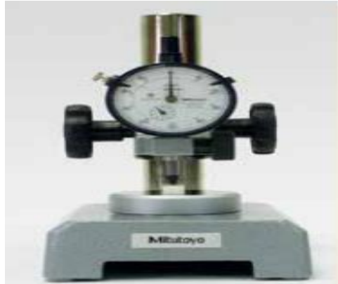
Fig.2.5. Zero setting with a 10 mm ceramic gauge block if the work piece nominal is 10 mm
