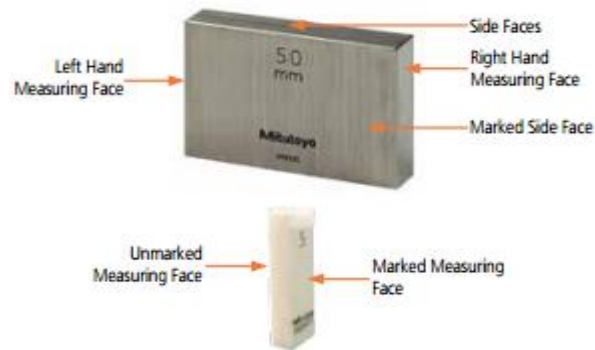
Fig. 2.59. parts of gauge block
