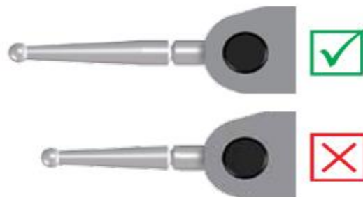
Fig.2.49. correct use of dial test indicator
