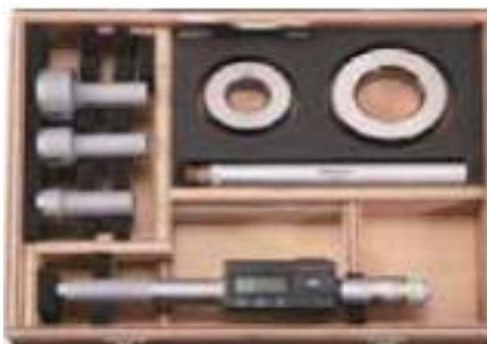
Fig.2.9. 3-point internal micrometers with exchangeable measuring heads
