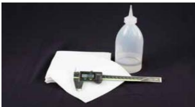
Fig.2.3. Remove dust or dirt from the measuring instrument
