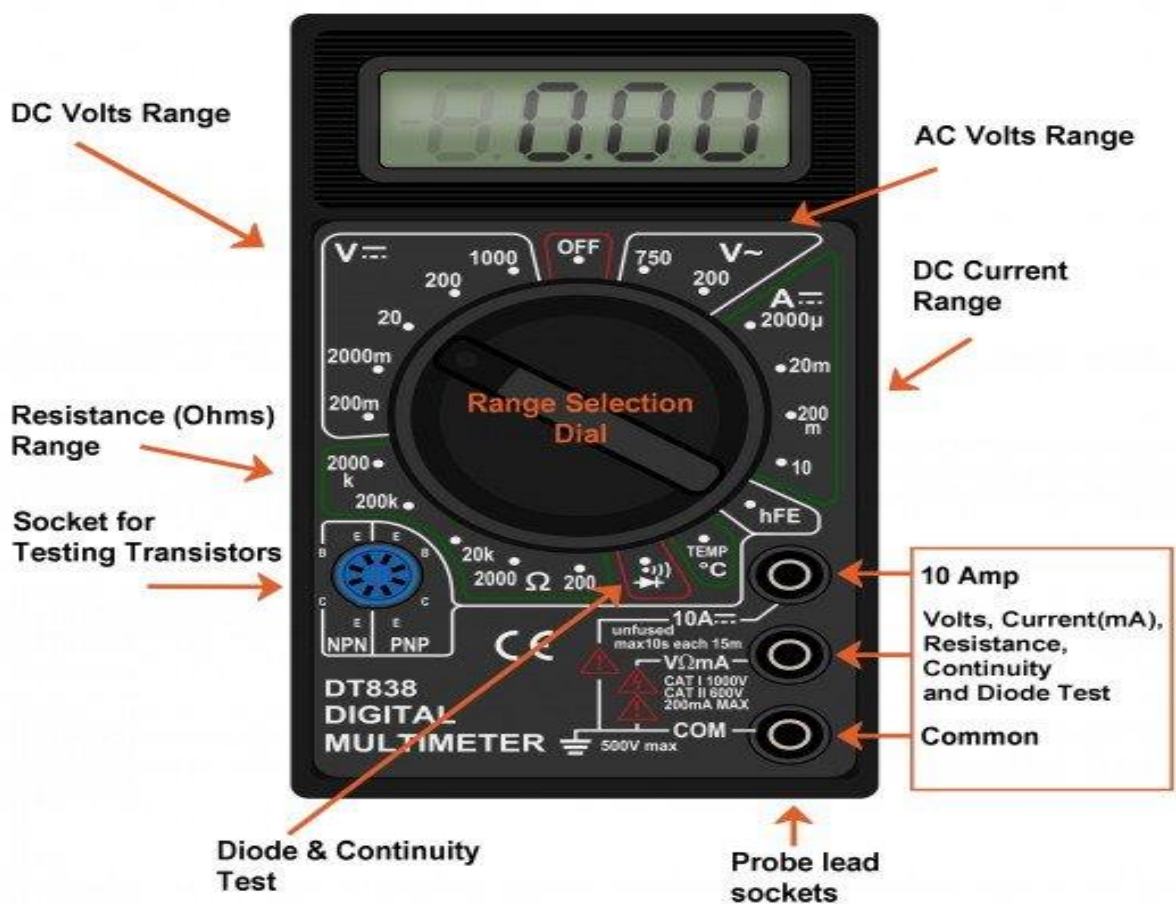
Figure1.5: Voltage, Current and Resistance Ranges
