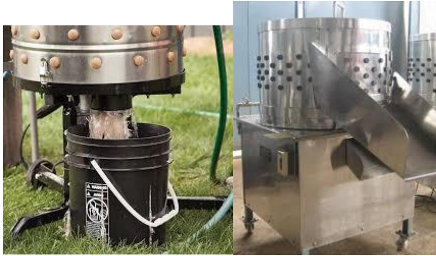
Figure1 Poultry de-fathering machine
