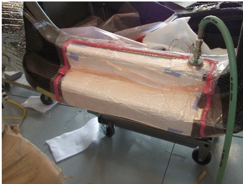
Figure 25: Vacuum-bagging the repair patch pulls out air bubbles from the uncured resin and also helps ensure a good bond.
