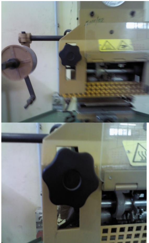
Micro switch that controls the going down of the printing group
