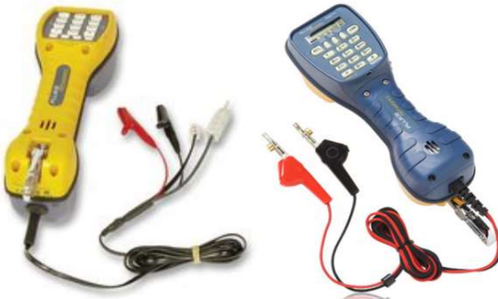
Fig 10. Pair Continuity tester
