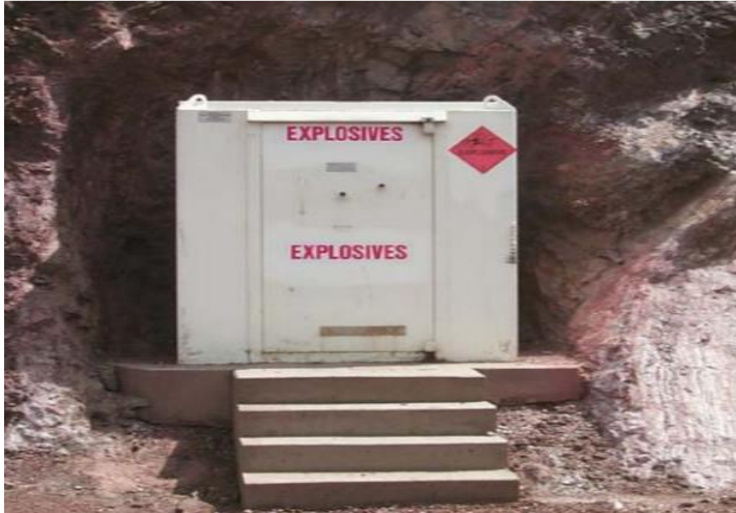
Figure 1: Relocatable magazine fixed to prevent unauthorized removal.
