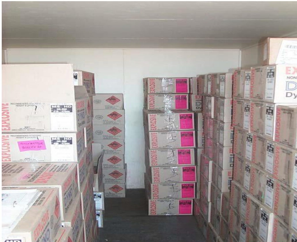
Figure 1: Explosives stacked with their labeling towards the access way for easy identification.
