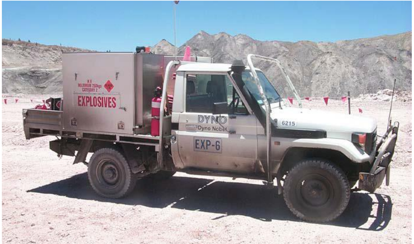
Figure : Explosives vehicle at a mine site with separate explosives receptacles and fire extinguishers.
