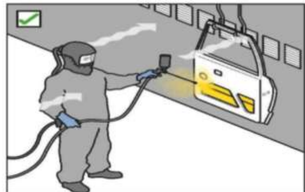
Figure 4 Spraying with a 'long' nozzle avoids overspray of the operator.
