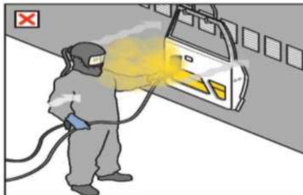
Figure 3 Spraying with a 'short' nozzle may cause overspray of the operator.
