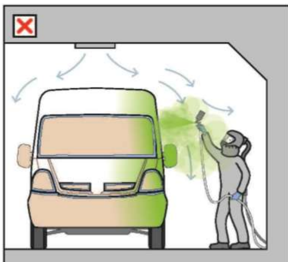
Figure 7 The operator is exposed to overspray and stretching and reaching can cause discomfort and injury.
