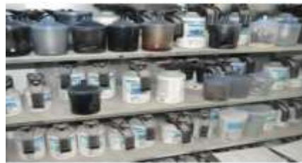
Fig:- Store and mix water-based paints only in plastic or inner-coated tin containers to avoid corrosion contamination problems.
