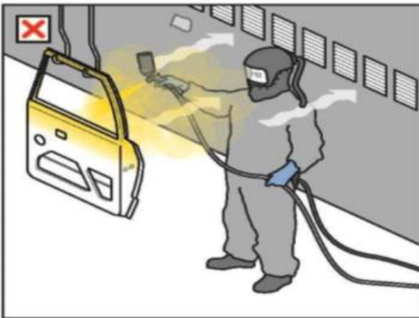
Figure 1 The operator is exposed to overspray because of poor positioning in relation to the airflow.
