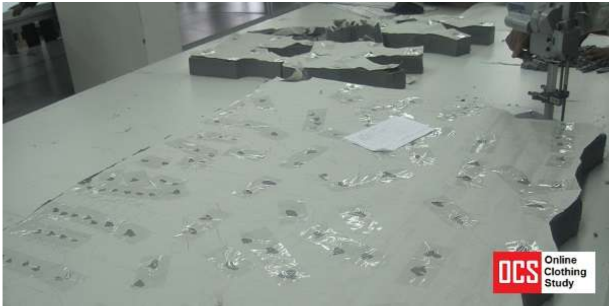
Figure 11: Bulk fabric cutting using a straight knife cutting machine
