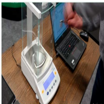
Figure. 10. Weighing scales Calibrating process showing images
