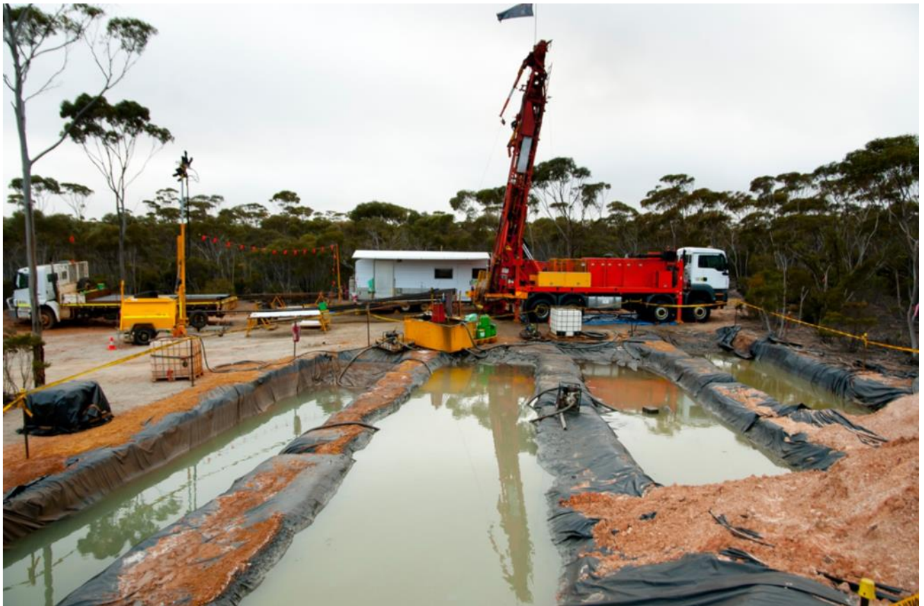
Fig 3: Reverse Circulation Drilling (RC)
