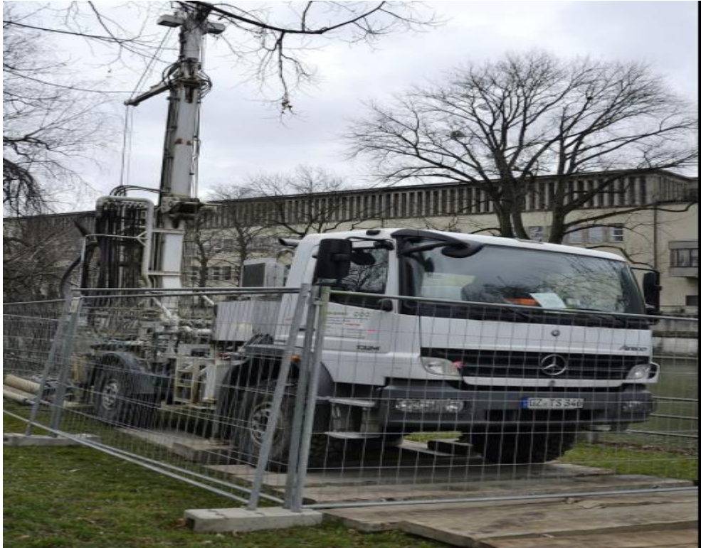
Fig 1: Mobile drilling rig mounted on a truck
