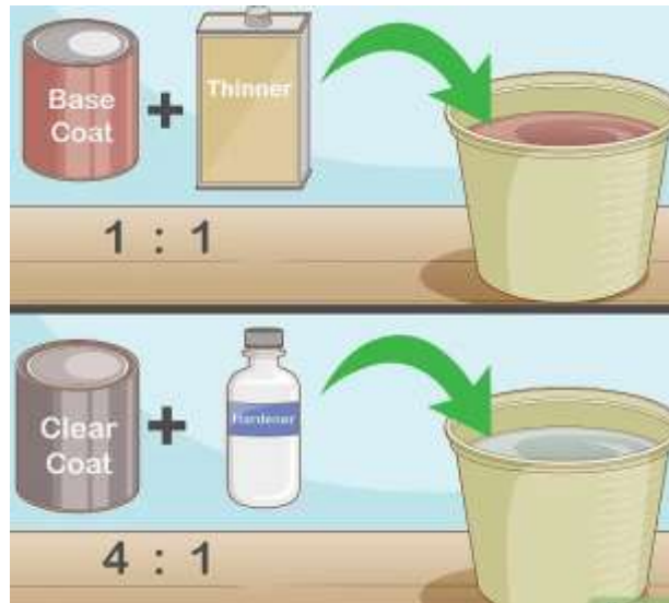
Figure 12. combining paint materials
