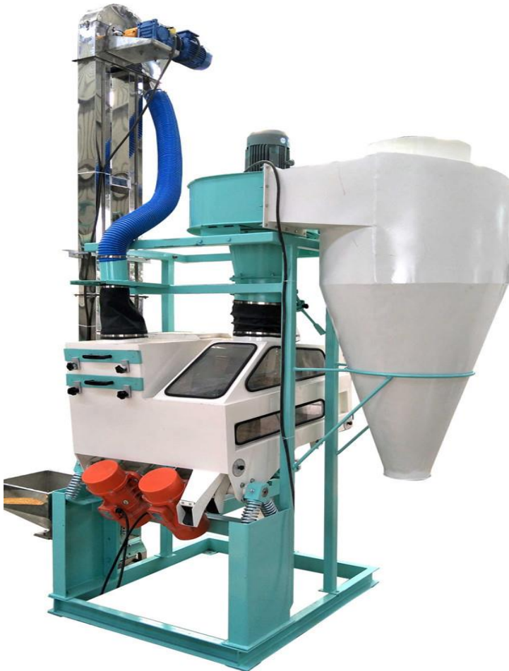
Figure 2.2: De-stoner with a vibratory sifter, bucket elevator and motors
