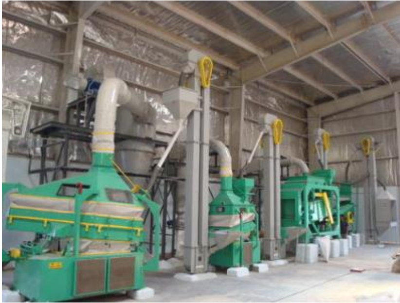
Figure 2.5: Vacuum gravity separator (air table)
