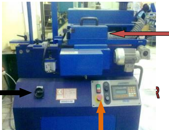
Shank Heel Length Gap Adjustment from Back Side
