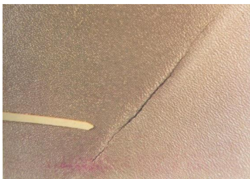
7. Fig2.9 Flay Cuts:- these flaying defects reduce considerably the value of a hide (skin). The damages can all be avoided since they are caused by carelessness or flaying by inexperienced person or by using improper tool.
