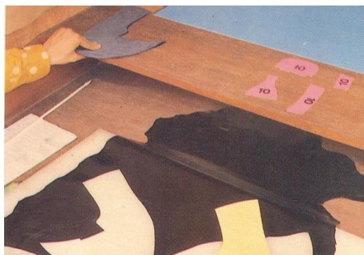
Figure 148: check cut component quality
