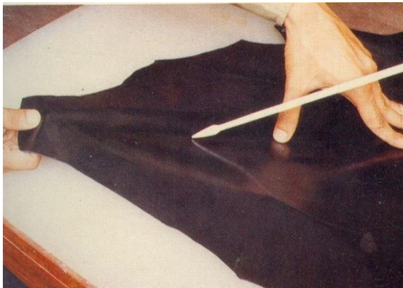
Figure 138: line of tightness
