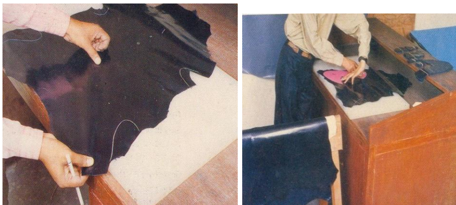
Figure 91: laying out leather
