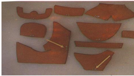
Figure 189. Laying grain side out and numbered
