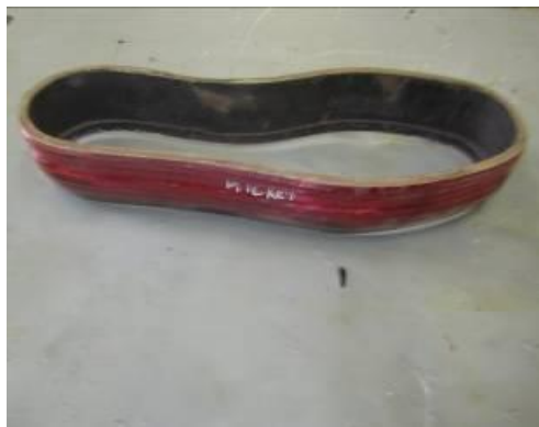
Figure 82: dies for insole board and Shank board Cutting
