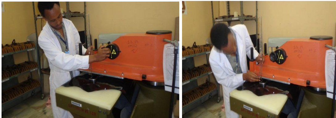
Figure 170: adjust pressure & height of the Aluminum plate
