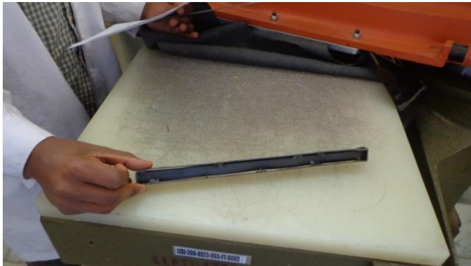
Figure 171: check the shape of the die
