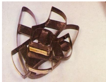
Figure 86: not placing dies on top of another
