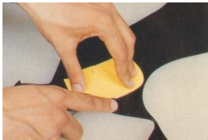
Figure 162: cut the single tongue
