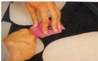
Figure 163: cut the tongue for the above pair
