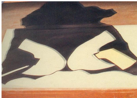
Figure 147: cutting the 3 rd left quarter
