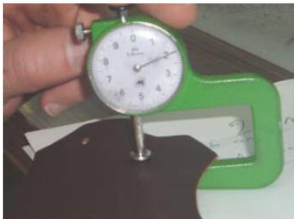
Figure 194 Checking the thickness
