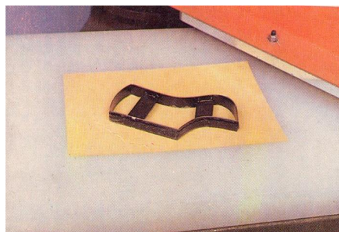
Figure 117: Placing the die on card board
