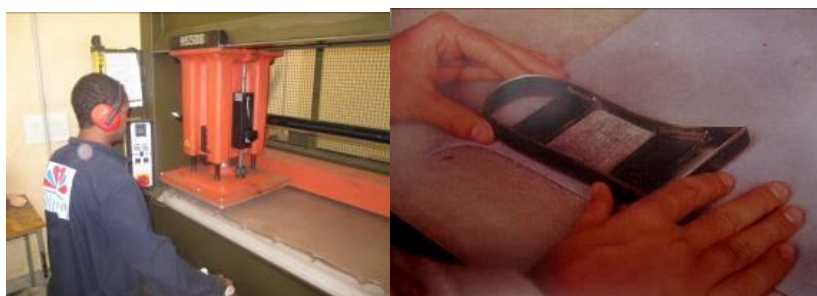
Figure 78: cutting shank board
