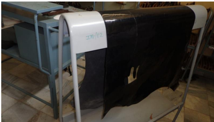
Figure 174: putting the leather on the leather horse
