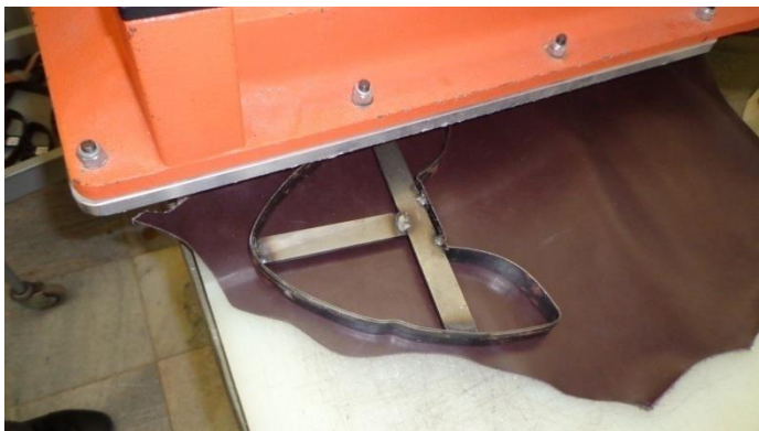
Figure 179: Cut large components first
