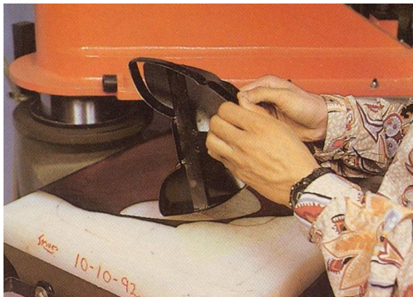
Figure 57: Picking up the cut and the knife
