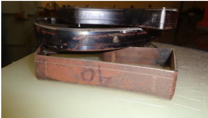
Figure 173: not keeping the dies on top of another
