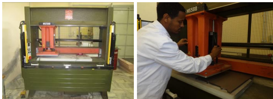
Figure 74: Travelling Head Clicking Press
