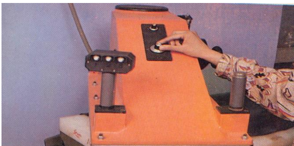
Figure 120: Adjusting the pressure
