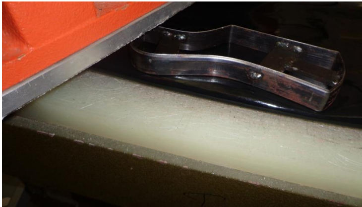
Figure 178: do not cut leather in layer
