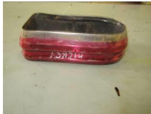
Figure 82: dies for insole board and Shank board Cutting
