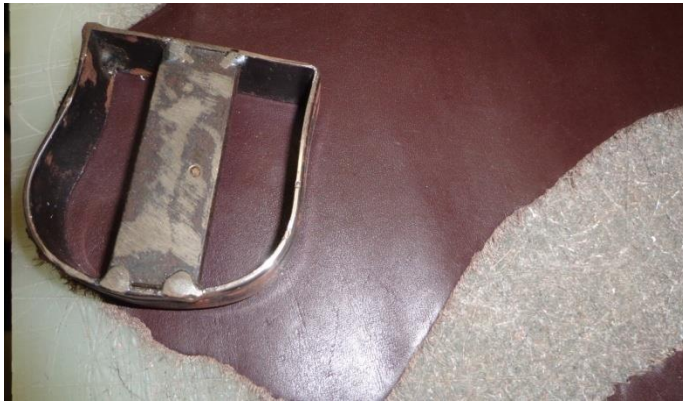
Figure 180: components cut edge to edge to minimize waste
