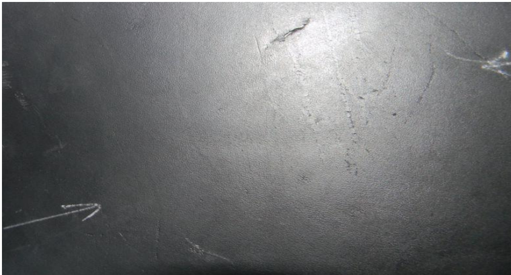
Figure 103: Scratches or Blemishes in the Grain
