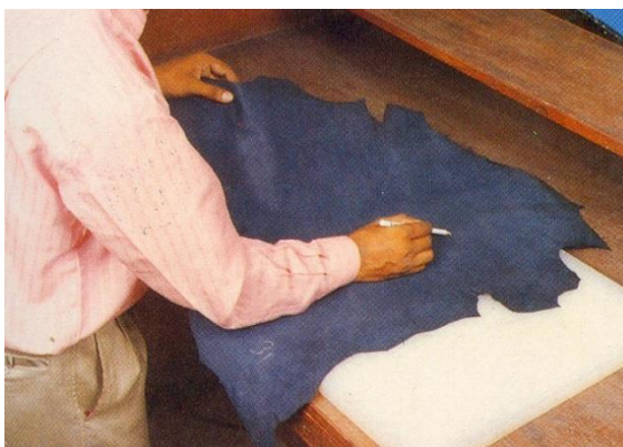
Figure 136: check flesh side for warble holes and flay cuts
