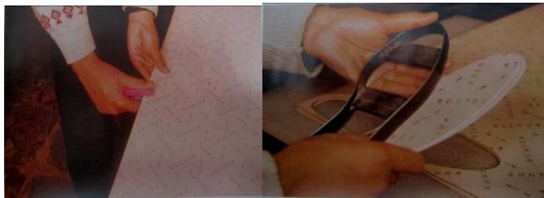
Figure 77: cutting insole board
