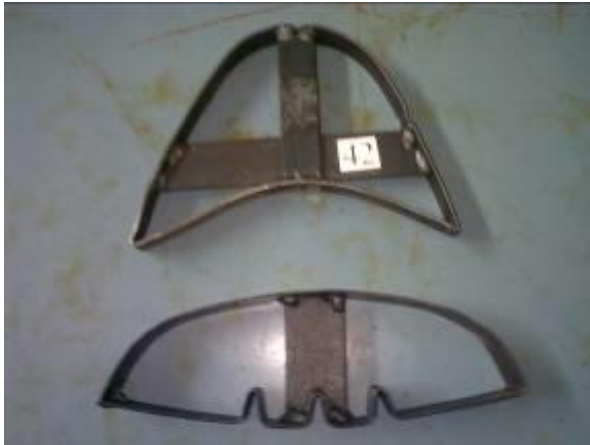
Figure 81: dies for Foam, Textile, Toe-puff and Counter Stiffener Cutting
