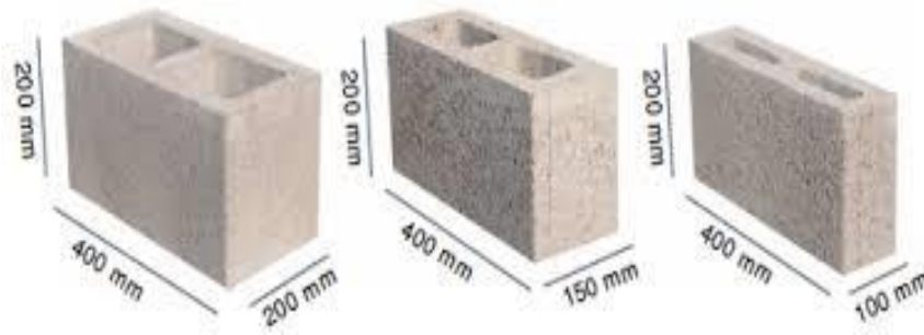
fig 5.1 standard dimension of hollow concrete block
