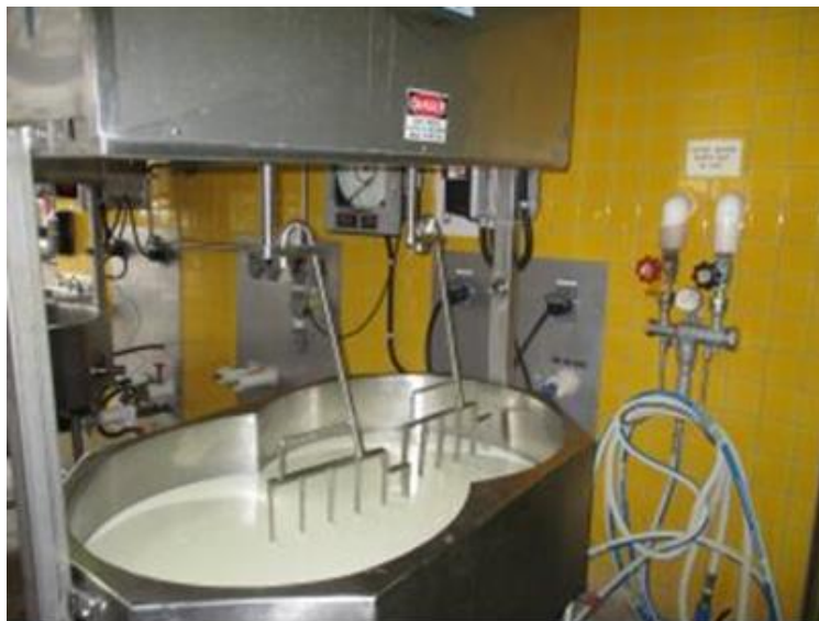
Figure 69: Automated cheese knives in a double 'o' vat.
