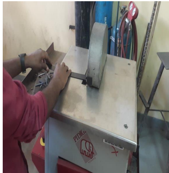
Figure : cutting steel rule
