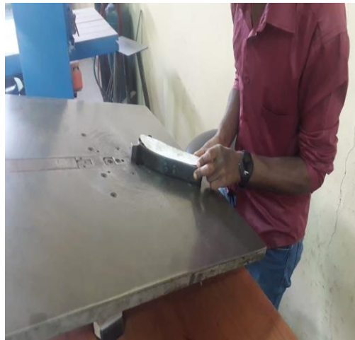
Figure : die bending process
