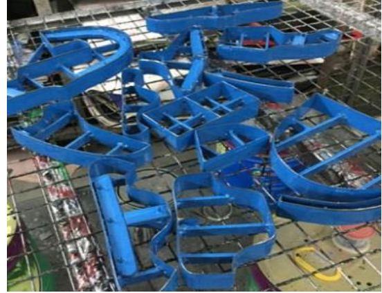
Figure 3. Cutting dies getting a coat of paint
