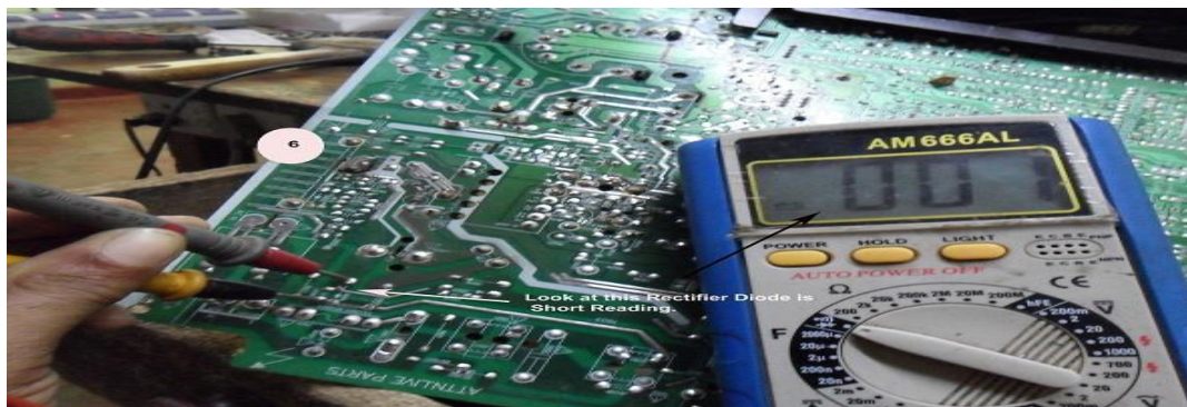
Fig 2.5 short circuit test
