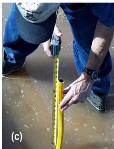
Figure 49: Demonstrating how to measure the “drop” in a surface system (a) Use the hose to siphon water out of the ditch; (b) Raise the hose up until water stops flowing out of the hose end; (c) Measure the distance between the end of the hose and the water level in the field.
