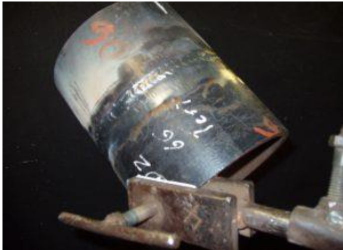
Fig5.5Side view of the hot pass
