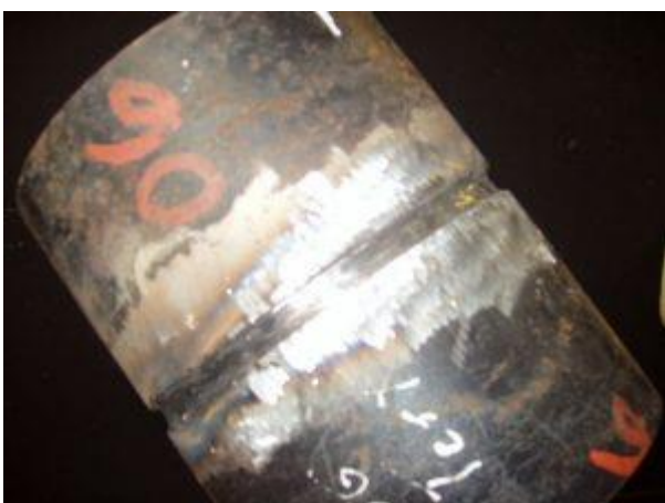
Fig5.4Top of the ground down root and this will be the base for the hot pass.
