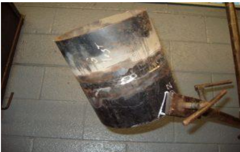
Fig5.3 a side view of the ground down root pass.
