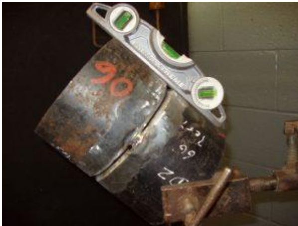
Fig 1.1 Checking the 6G pipe test to make sure it is at a 45 degrees with a magnetic level
