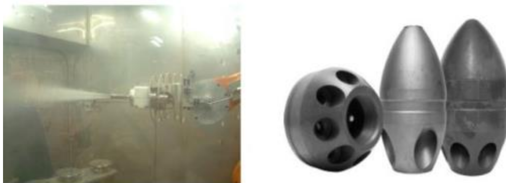
Figure 1: Flushing Operation and Different Nozzles
