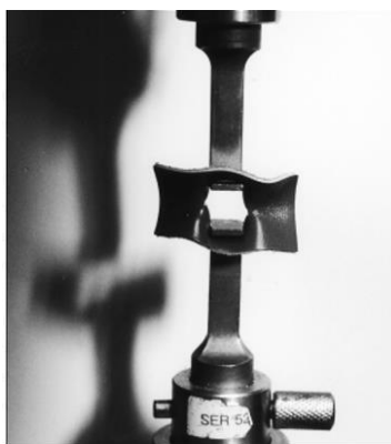
Double edge tear test grip of leather
