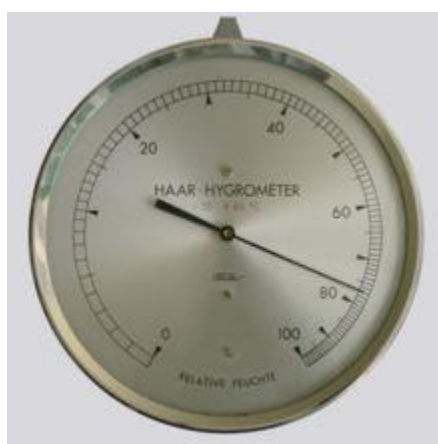
A hair tension dials hygrometer with a nonlinear scale
