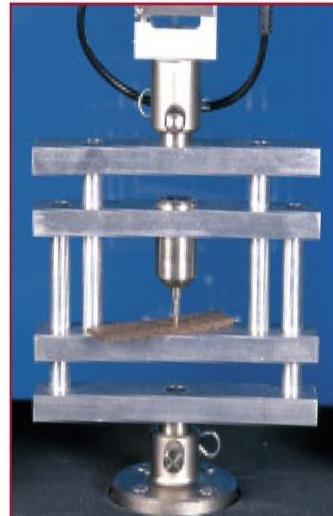
Insole pin holding strength
