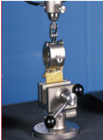
Sole bond test grip test
