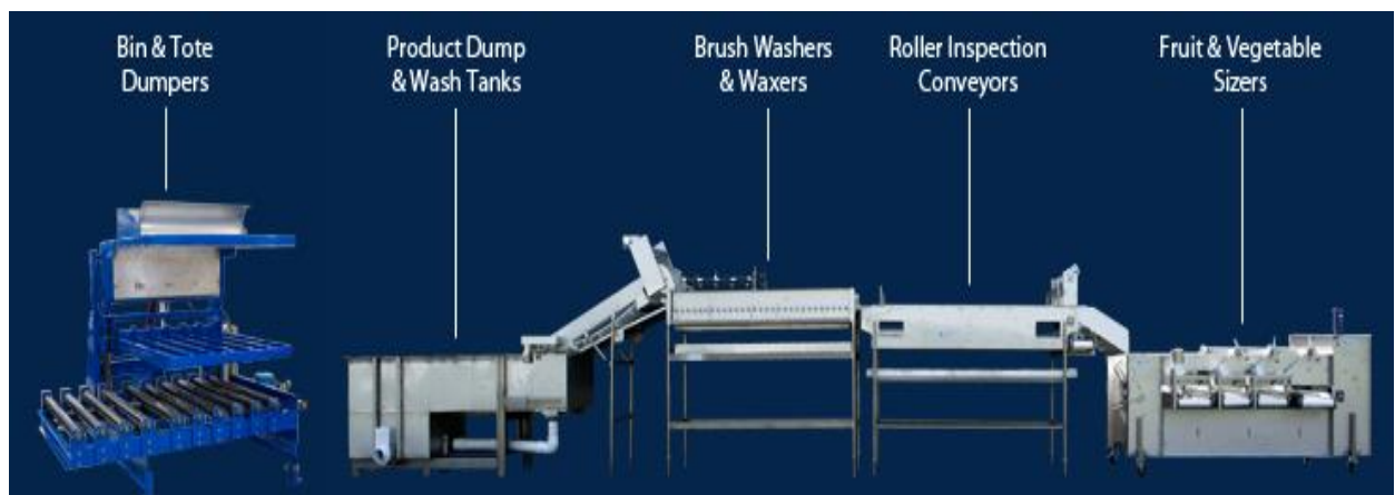
Figure 10 : Cleaning, sorting and grading line
