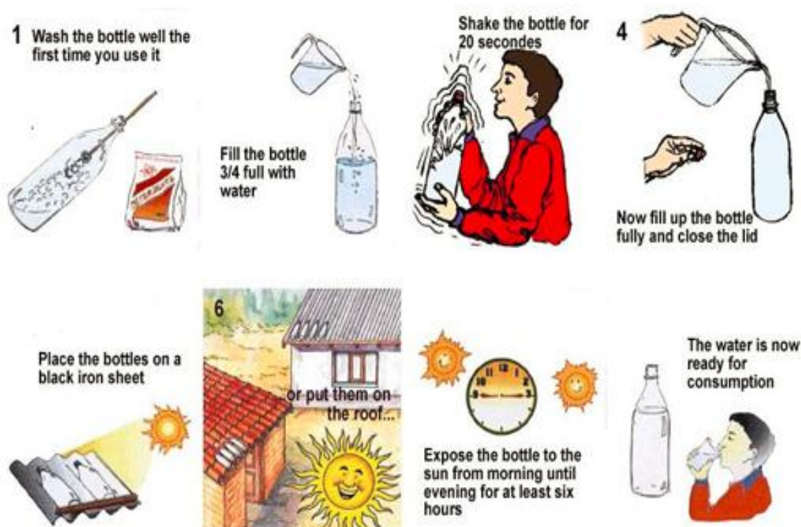
Figure 21: The procedures for solar disinfection of water (SODIS)
