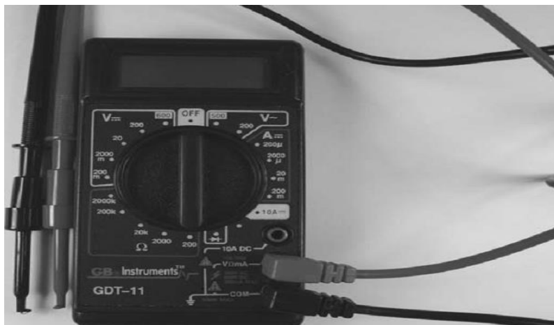
Figure 2 A multimeter is a measuring device that you'll use often.
