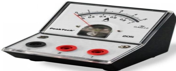
Ammeter, e.g. Galvanometer or Milli Ammeter (Measures current)
