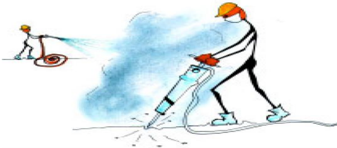
Figure 5.1. Use water to suppress dust and/or wear a dust mask.
