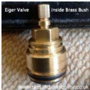
Fig :6.10 Example of Valve stuck inside Brass Bush
