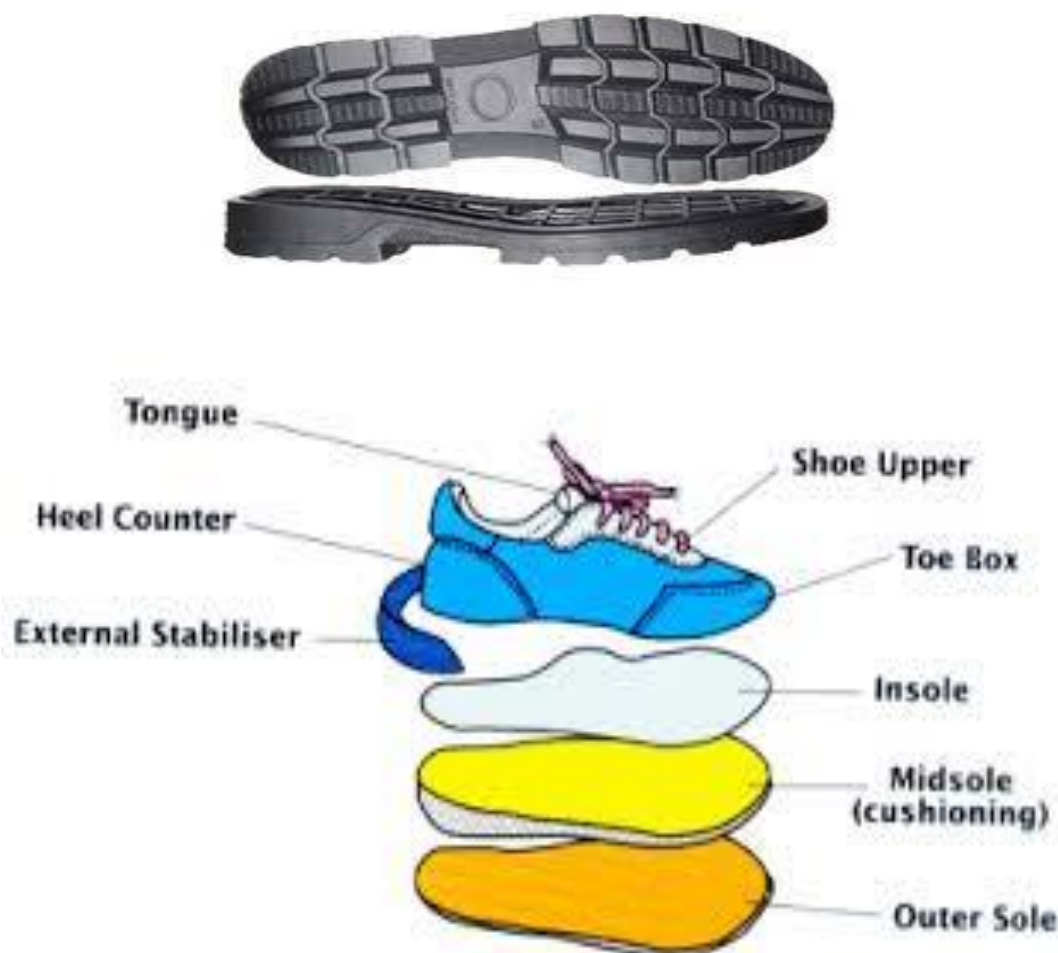
Figure 55 Soles and midsoles
