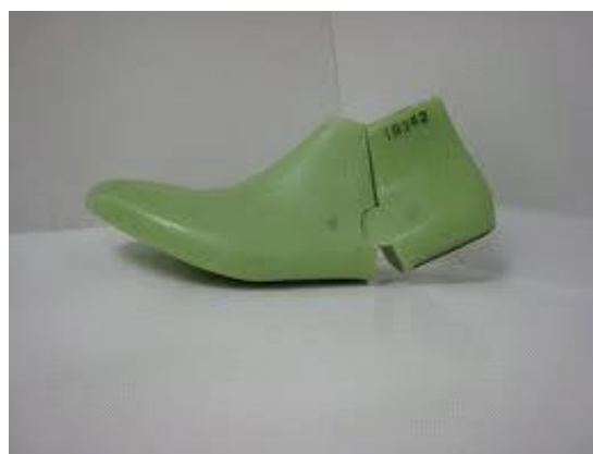
Figure 40 V- hinge last
