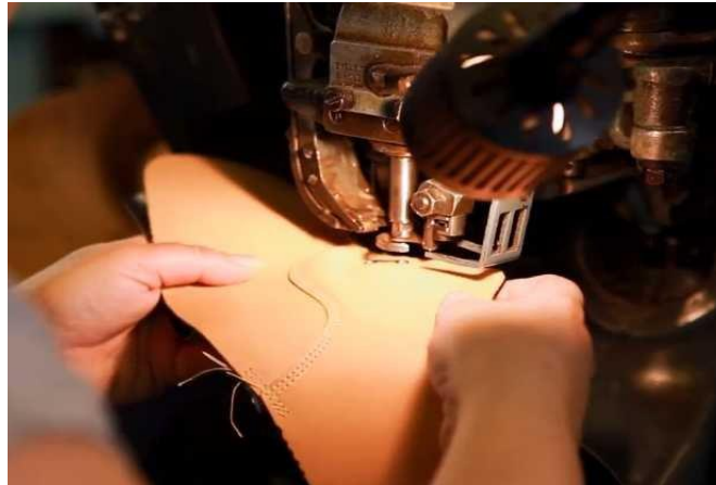
Figure 26 in the closing room, the cut pieces of leather are assembled and stitched
