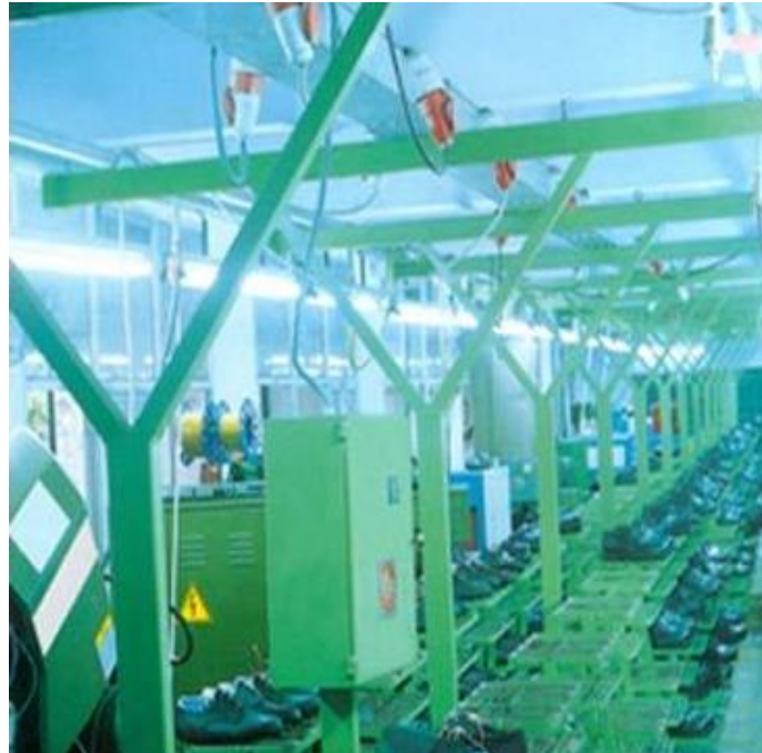
Figure 32 A mechanized footwear conveyor
