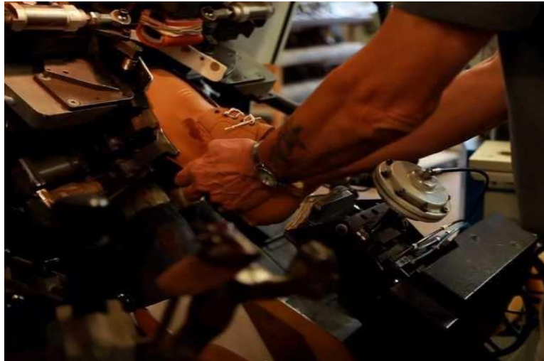
Figure 27 the shoe is listed on the top sides by a fore-part lasting machine
