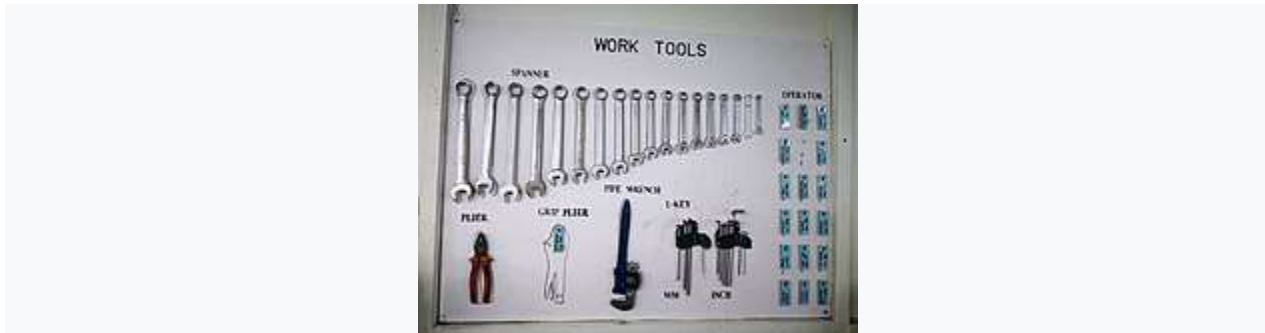
Figure 3.4. Shadow Board (with tools' outline) and worker's movement that is being used in Production floor
