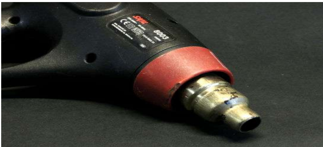
Figure 1.4.Heat gun: very efficient but unselective
