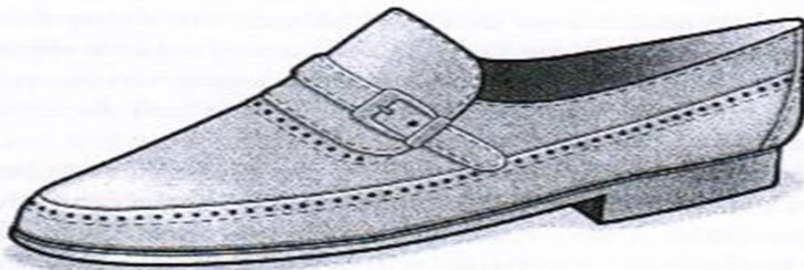
Figure 4.9 Line drawing of a buckle and bar arrangement to a high-vamp shoe. (Reproduced with permission of Rossi & Tennant 1993.)
