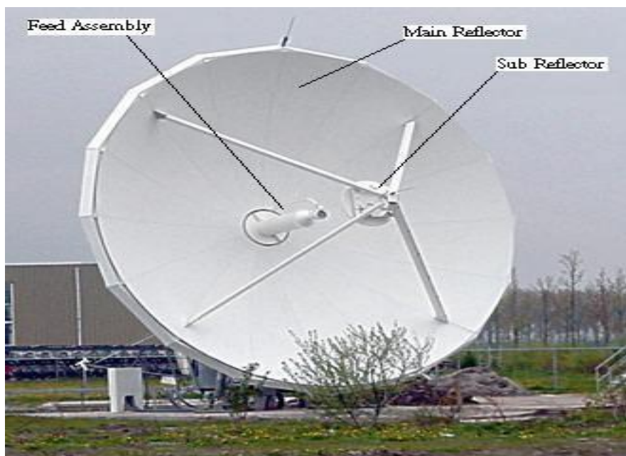
Figure 2.2: Parts of Dish Antenna
