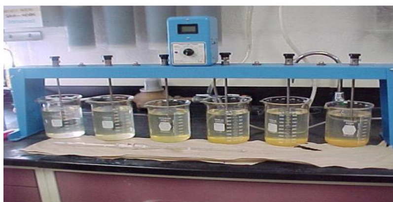
Figure. 23 Jar Test set-up for PH
