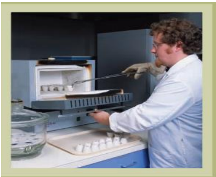
Figure. 12 High temperature incineration measure mineral (ash) content
