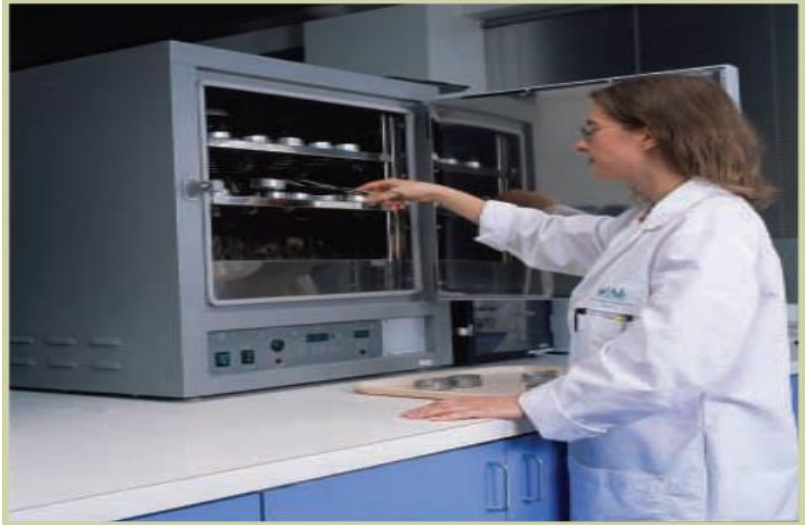
Figure.10 Low temperature heating to measure moisture content
