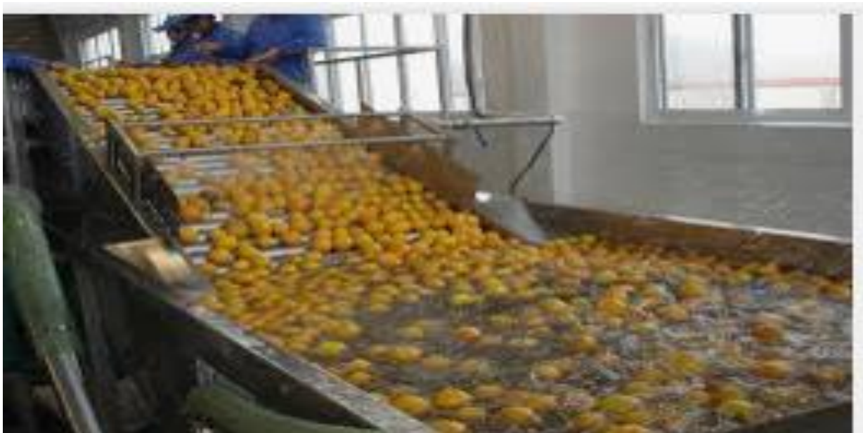
Figure3: fruit washer and conveyer belt
