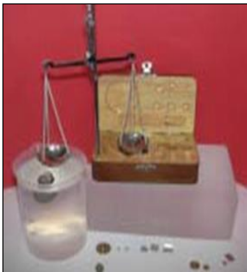
Figure 4: Determination of the weight of a sample
