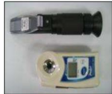
Refractometer, analog (top) and digital (bottom)
