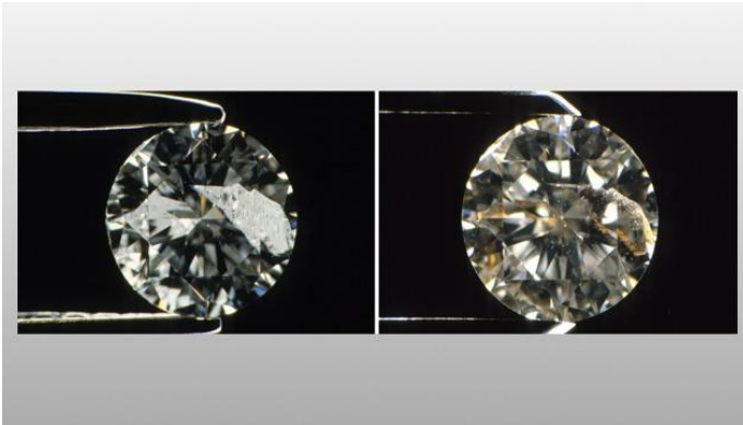
Figure 60. Surface reaching fractures in diamonds can be filled with molten lead glass, lessening the appearance of the fractures.
