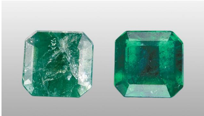
Figure 62. Surface reaching fractures in emeralds, such as this one can be filled with artificial resins, wax, and epoxy polymers. This lessens the appearance of the fractures, as the treated emerald on the right shows.
