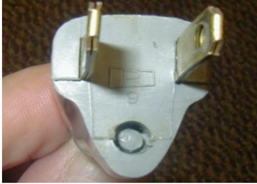
Figure 1.3 Three Prong Plug Missing Ground
