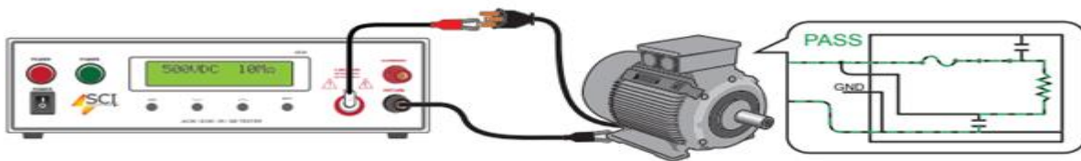
Figure 8.4 insulation resistance testing of motor
