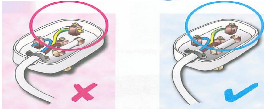
Figure 3.2 wiring the cord of electrical equipment to a plug
