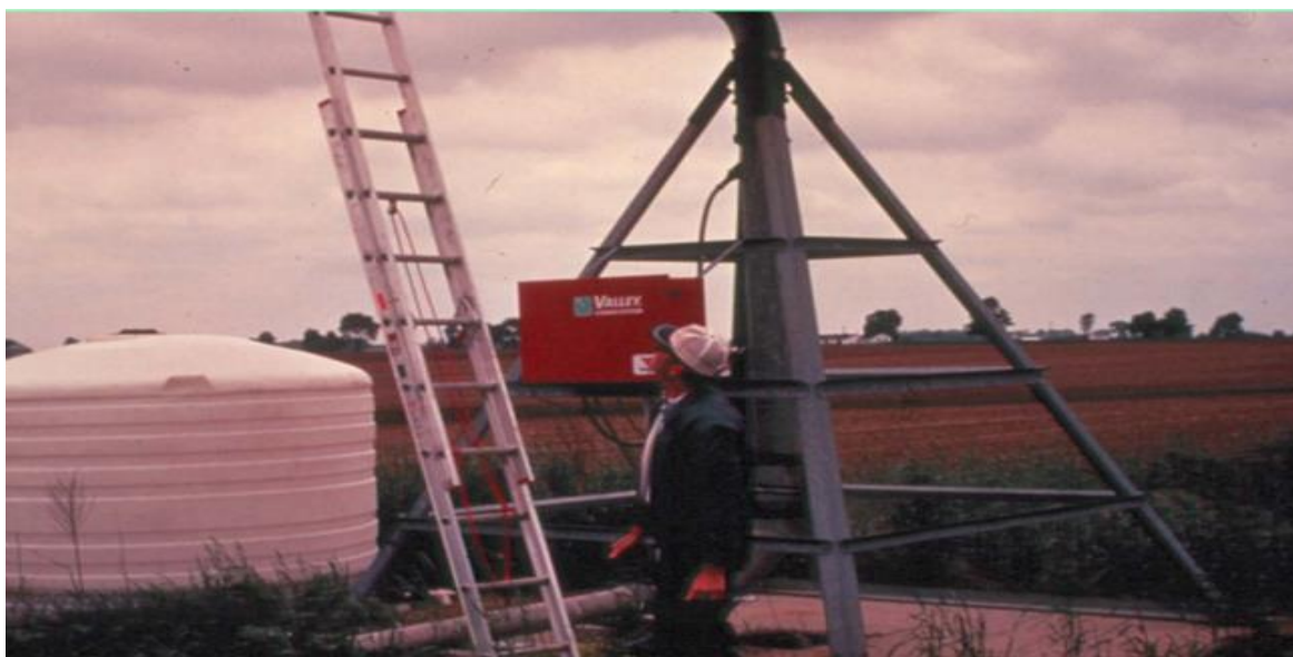
Figure 1: Use a good ladder or stable lift device to perform overhead repair and maintenance on an irrigation machine.
