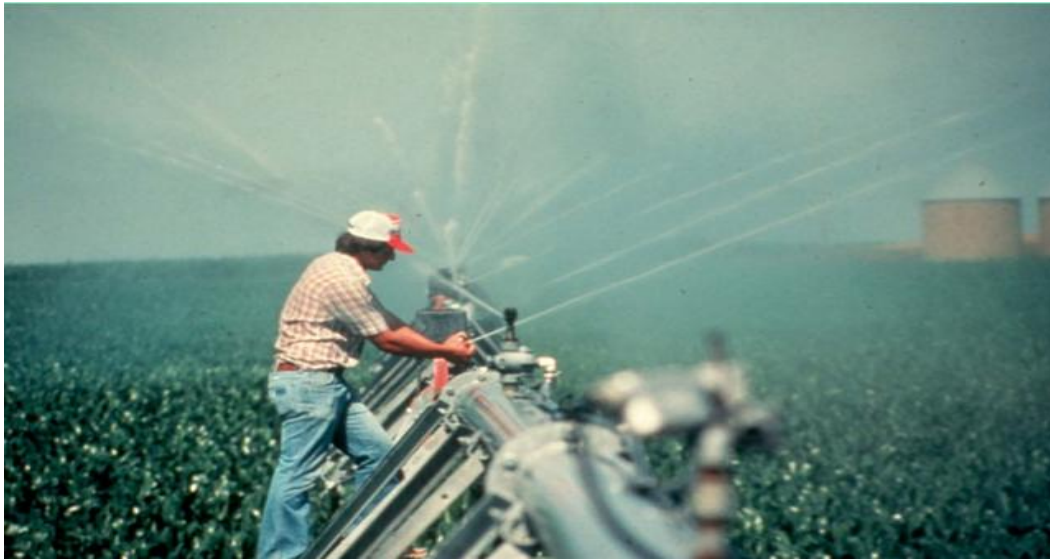
Figure 2: High pressure water jets can cause physical harm, especially to eyes, and can also cause falls from irrigation systems.
