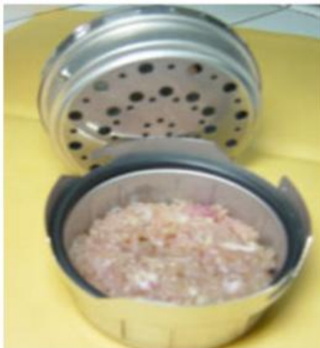
Figure-26 Aw-meter with product sample to be tested, lid (has to be attached) with built-in hygrometer
