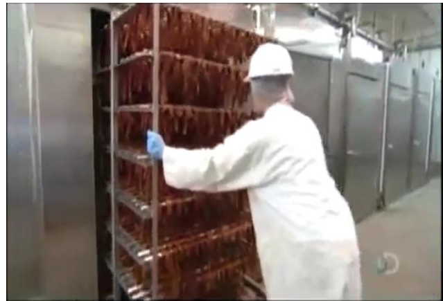
Figure 15a loading sliced meat on metal rode Figure 15b loading meat in to drier
