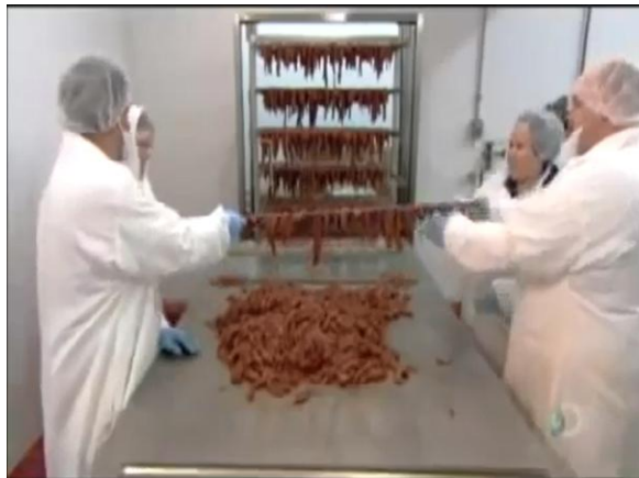
Figure 15a loading sliced meat on metal rode Figure 15b loading meat in to drier
