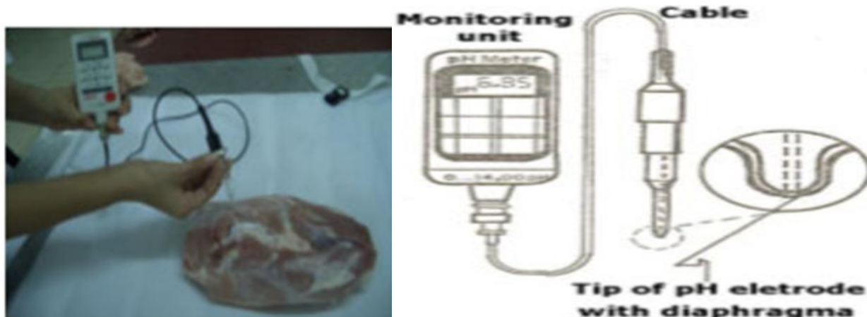
Figure25. PH meter & pH meter. Inserting glass electrode in meat tissue
