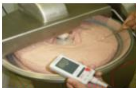
Step 5: The mixture is finely chopped until +12°C is reached
