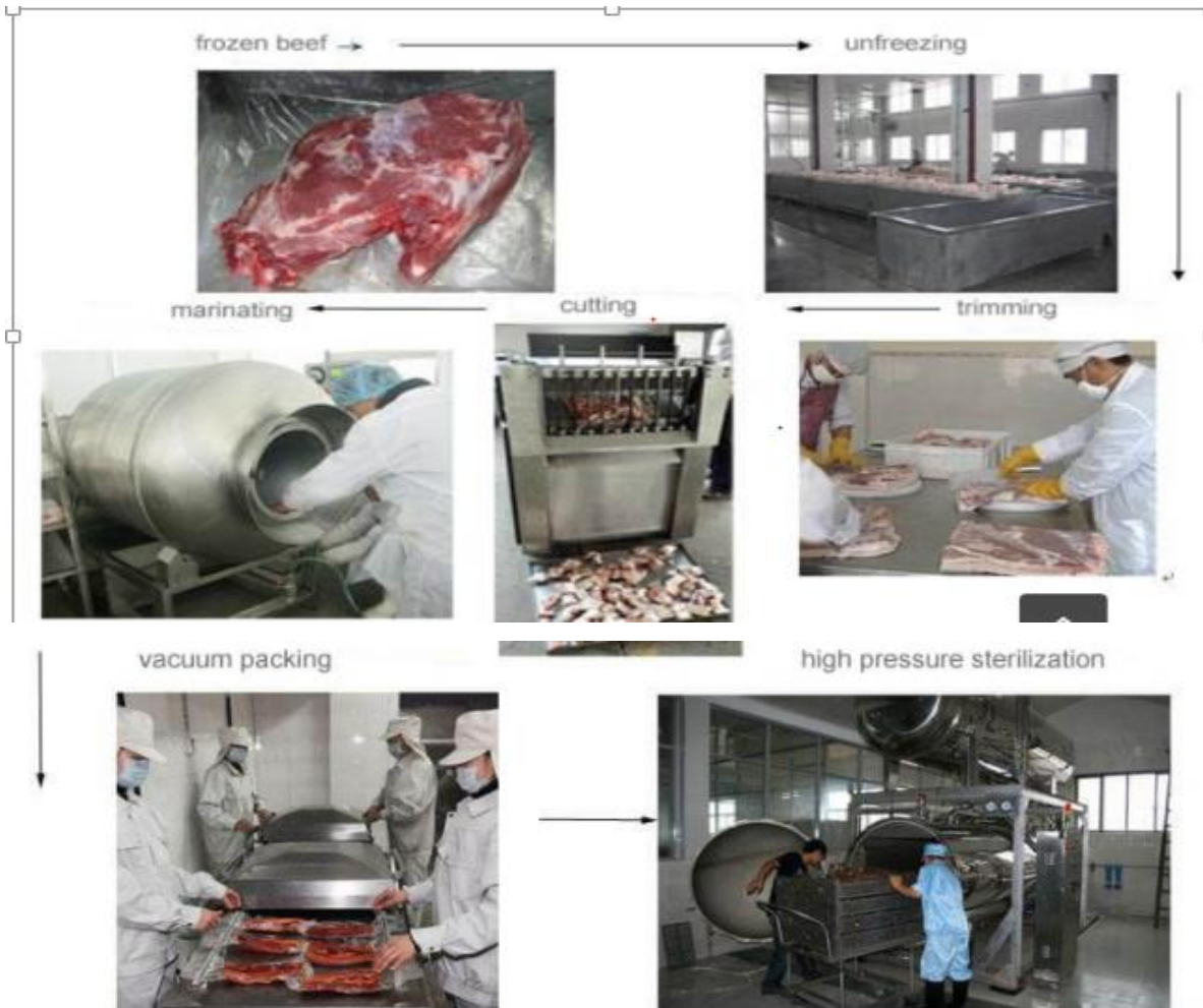
Figure 30. Corned beef processing flow and equipment
