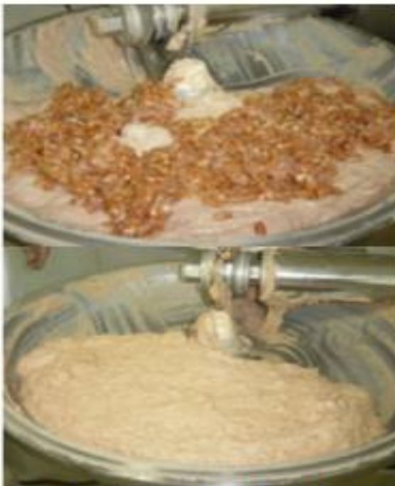
Step 2: Coarse material is added to finely chopped batter (above). Final mixture after a few rounds in the bowl cutter (below)
