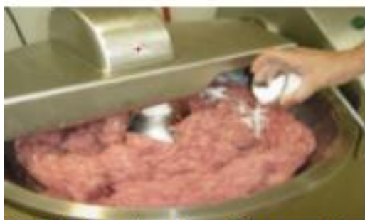
Step 2: Dry-chopping of lean meat, curing salt and phosphates
