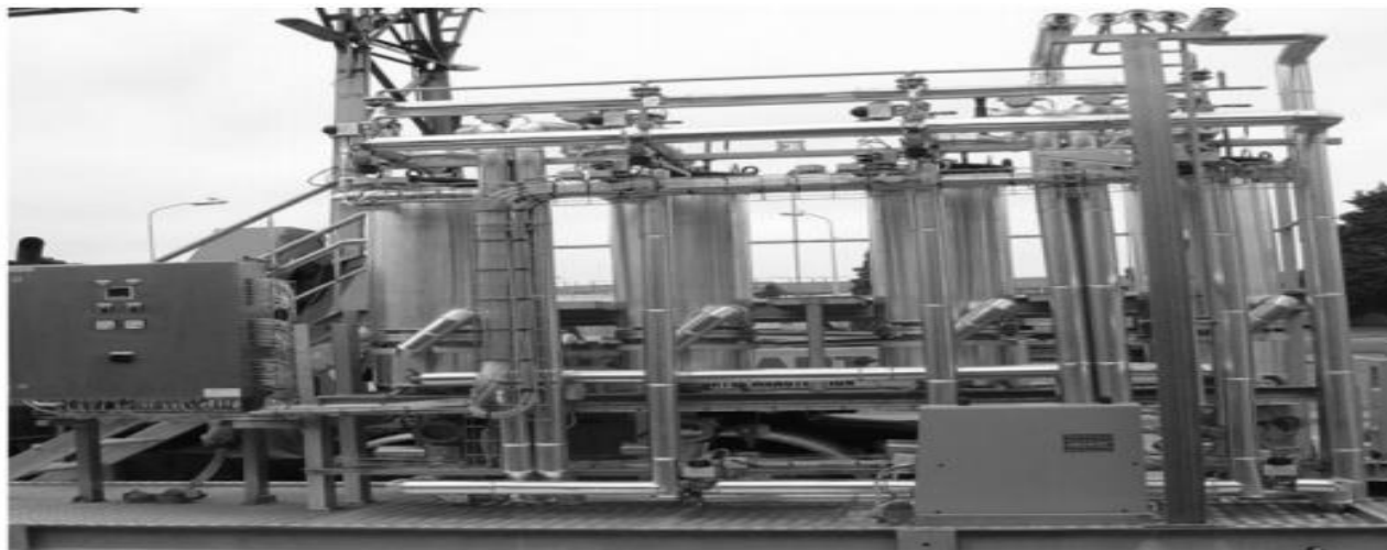
Figure20 Industrial enzymatic interesterification plant (four packed-bed reactors)
