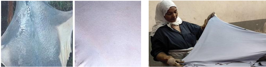
Figure 5.1: Grading of pickle pelt and wet blue leather
