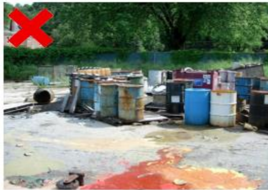
Fig. 3.6: Bad storage condition of chemicals
