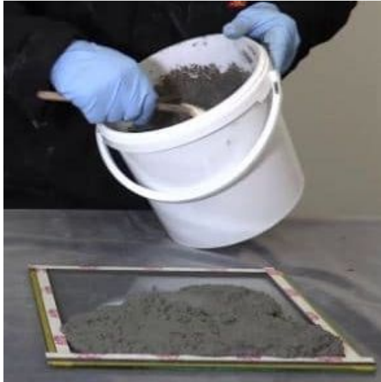
Fig3.2: Latex Modified Mortar
